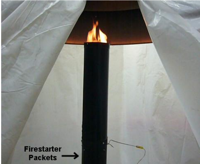
Figure 2. Simulated chimney fire, run 2
